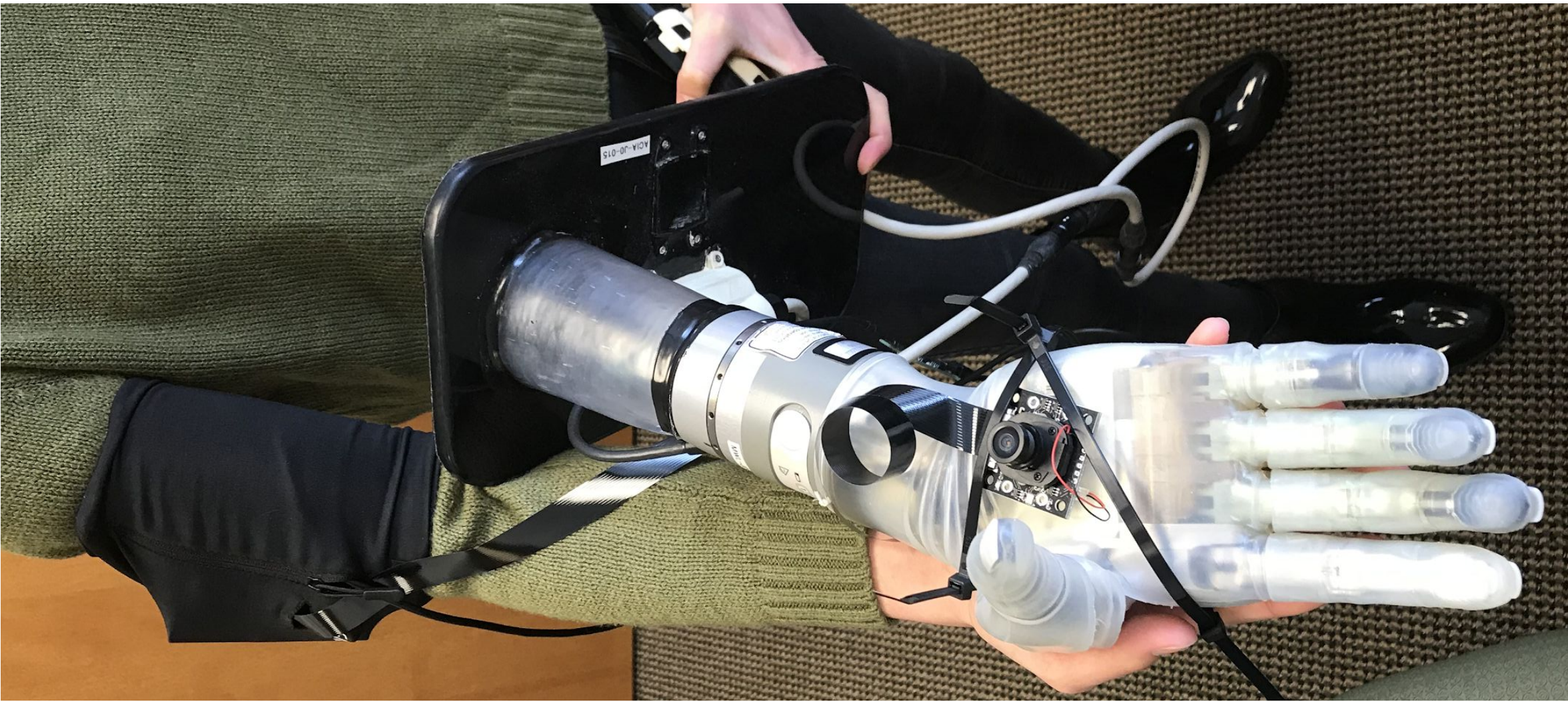
Current Prototype: The camera mounts to the heel of the DEKA hand and sends image data to the Raspberry Pi (encased in the armband with its battery). The Raspberry Pi sends grasp commands to the DEKA hand.
